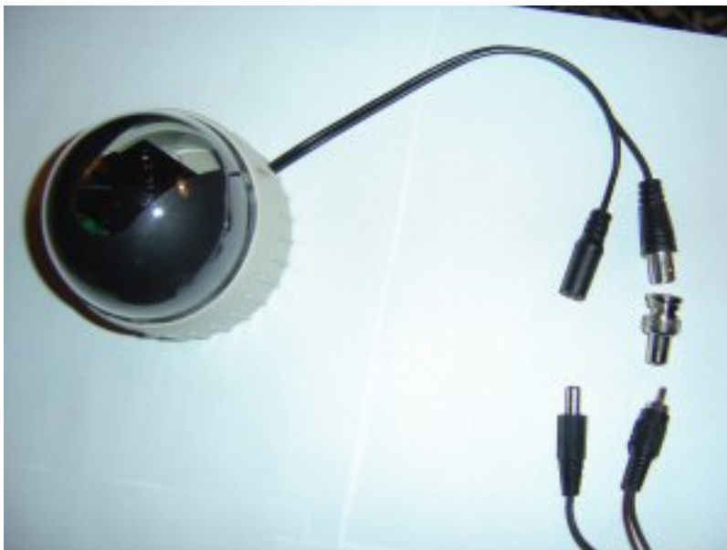
Figure 2-E CCD Camera with BNC shown laid out before connecting cable Note: Cables would normally be routed inside the wall with a Dome camera, shown for instructional purposes only.
