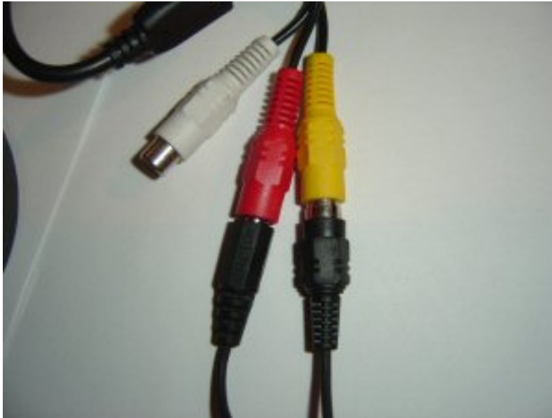
Figure 2-B Video (Yellow) and Power (Red) cables from camera plugged into All-In-One Cable Note: White cable used only for Audio (would require additional Cables)
