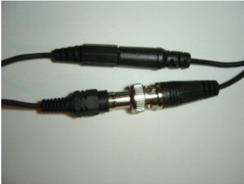
Figure 2-D BNC to RCA Adapter installed in Video Wire (Bottom)
